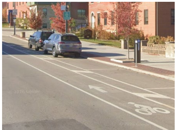
Akron examples of parking by the curb and bicycle lanes to the left: E. Market Street (left) and W. Exchange Street (right). Note the 3' striped buffer between parking and the bicycle lane
