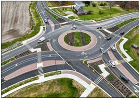
roundabouts is larger. FHWA is no longer recommending 2 x 2 roundabouts in many situations. However, 2 x 1 roundabouts—those where the higher volume road has two lanes, but the other street has single-lane entrances—have been much more successful. They can effectively handle capacity of high-volume roadways, particularly in suburban settings.
