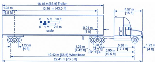
*WB-20 semi-trailers (53' trailers) require a large turning path.*
