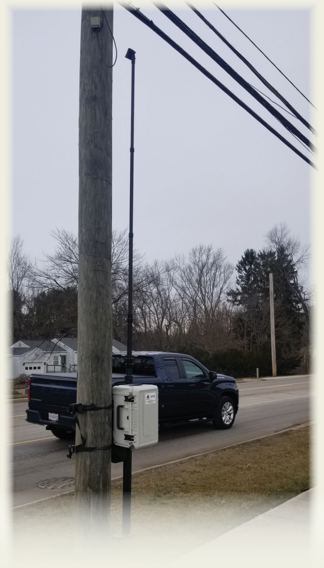
One of AMATS' miovision Scout Plus units deployed in the field to collect two-way traffic data.
